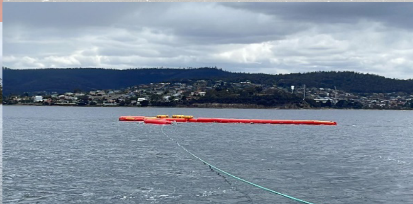
General purpose inflatable boom deployment
