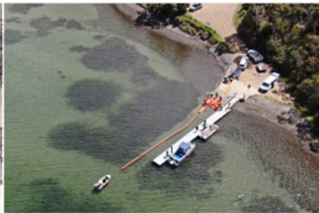
Deployment of general purpose inflatable boom
