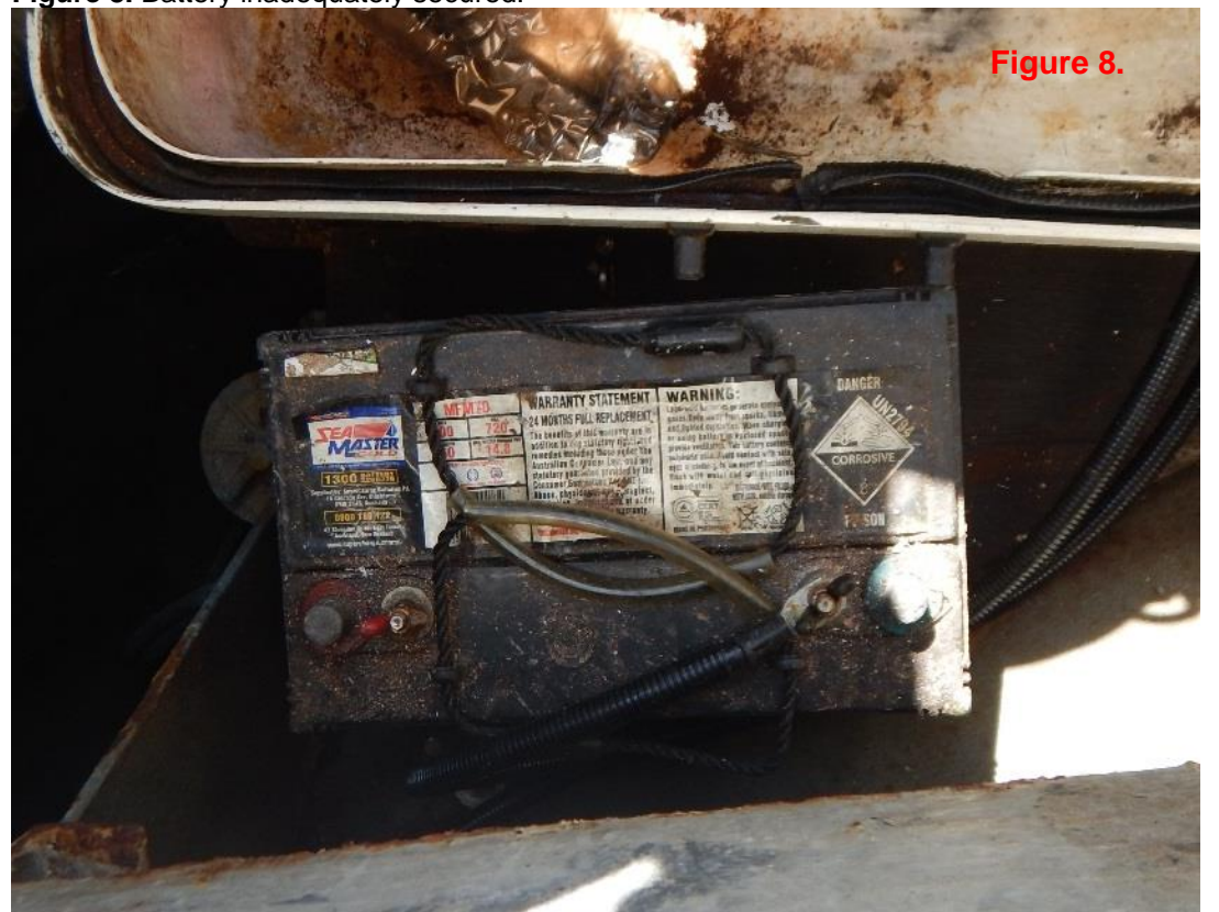
Figure 8. Battery inadequately secured.
