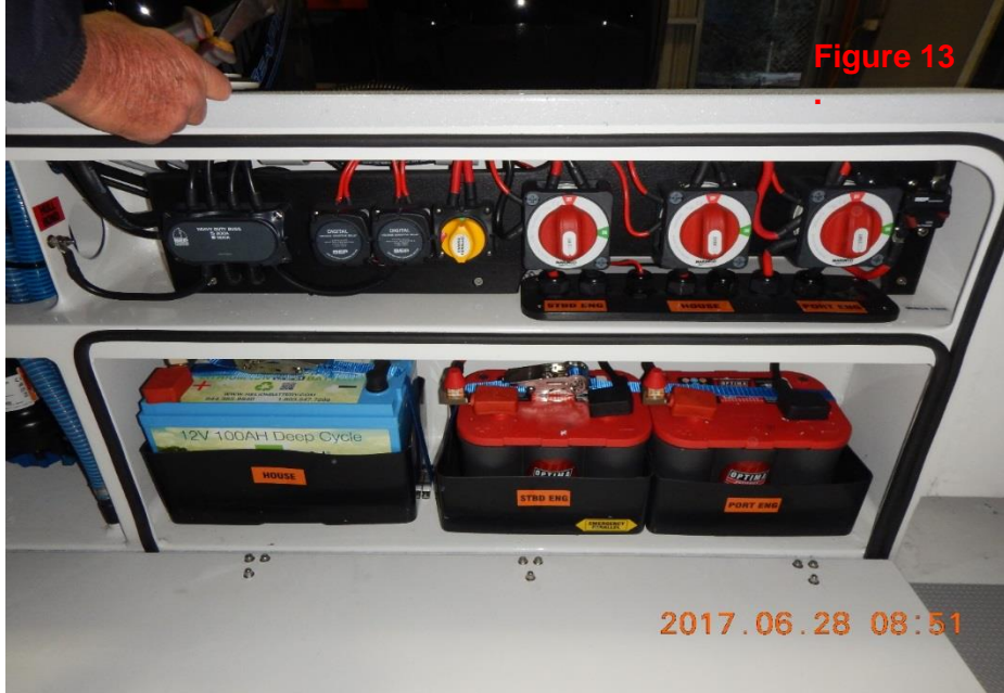
Figure 13. Batteries in this installation are separate from the switchgear. Wiring is routed through the panel via watertight/gastight glands. The door has ventilation. All components are labelled.
